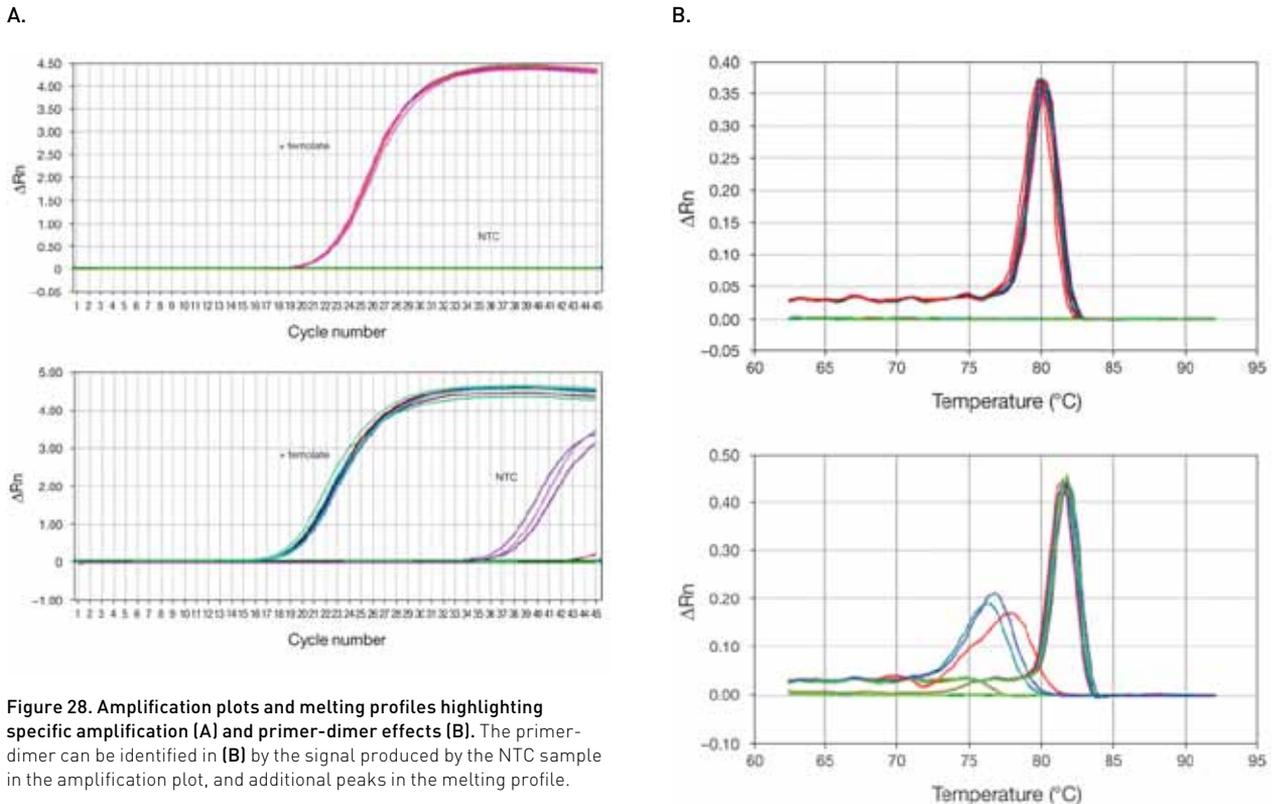
**Figure 28. Amplification plots and melting profiles highlighting specific amplification (A) and primer-dimer effects (B).** The primer-dimer can be identified in (B) by the signal produced by the NTC sample in the amplification plot, and additional peaks in the melting profile.
