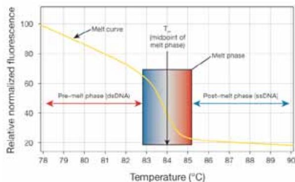
**Figure 27. Characteristics of the melt curve profile for a PCR amplicon.** Specific DNA sequences have characteristic melt-curve profiles. Mutations can be detected as either a shift in  $T_m$  or a change in shape of the melt curve. In contrast to traditional melt curve analysis, HRM can distinguish between amplicons with just a single-nucleotide difference. This technique has opened the door to many new applications for dsDNA-binding dyes.
