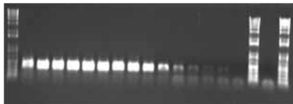
**Figure 16. Agarose gel analysis to investigate primer-dimer formation.** Prior to the thermal cycling reaction, the nucleic acid sample was serially diluted and added to the components of a PCR mix, and the same volume from each mixture was loaded on an agarose gel. Primer-dimers appear as diffuse bands at the bottom of the gel.
