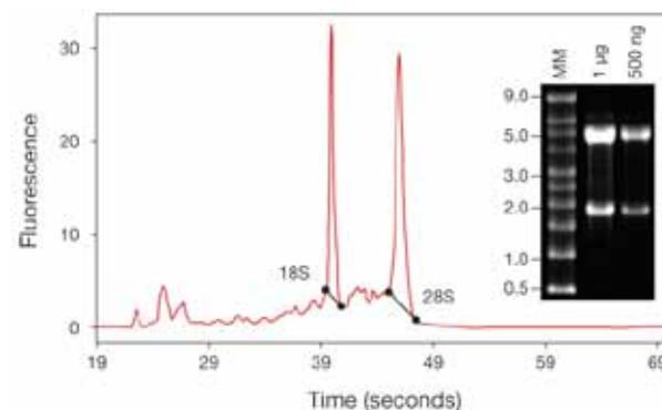
**Figure 17. Agilent Bioanalyzer trace and gel image displaying RNA integrity.** The two peaks in fluorescence correspond to the 18S and 28S rRNA bands. Intact mammalian total RNA shows two bands or peaks representing the 18S and 28S rRNA species. In general, the 28S rRNA is twice as bright (or has twice the area under the peak in the Bioanalyzer trace) as the 18S rRNA.
