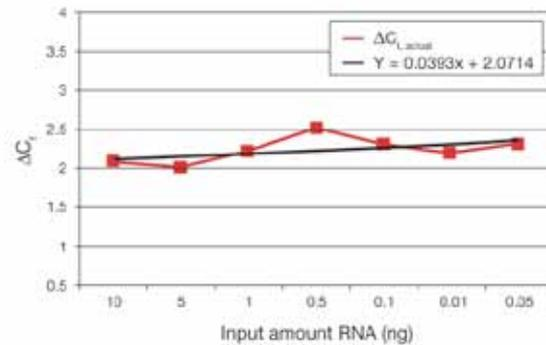
**Figure 25. Relative efficiency plot.** The  $\Delta C_t$  ranges from 2.0 to 2.5. When plotted against dilution or input amount of RNA, a slope is obtained. While a perfectly flat line (slope = 0) indicates identical efficiency across all input concentrations, a slope of <0.1 is generally considered acceptable when employing the  $\Delta\Delta C_t$  method.
