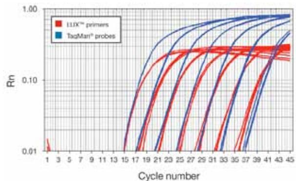
**Figure 33. Log plot screen shot showing an example of two sets of curves with differing plateau heights and therefore different exponential phases.** The most accurate portion of an amplification curve for  $C_s$  determination is directly in the middle of the exponential phase when viewing the log plot. The ideal threshold setting is sometimes unique for each set of data.
