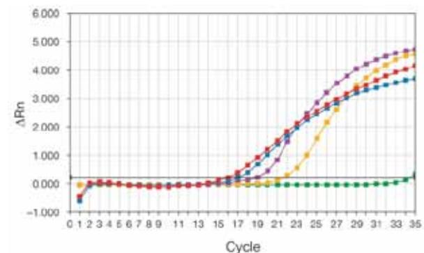
**Figure 30. Template dilution series to assess reaction efficiency.** Dilutions with earlier  $C_t$ s exhibit compressed  $C_t$ s and abnormal curve shapes. As the template becomes more dilute, inhibition vanishes and the curves take on the more characteristic exponential phase shape.
